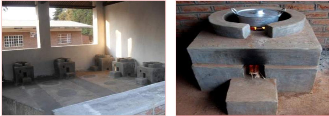
Top: Esperanza stoves at St Annes Health Centre, Bembeke – Dedza. Bottom: Esperanza stove in a home
