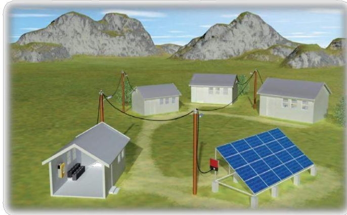
Image of a standalone solar mini grid System Source: SMA Solar Technology, Technology Compendium 2
